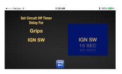
set this tap the "Off Timer Setting" box and another scroll wheel will appear. Here you have a choice of "ignition", which means the circuit will shut down when the ignition is shut off, or you
