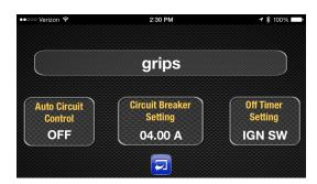
you shut off the ignition and then restart, the circuit will be in the off state. If you set memory to be on the circuit will revert to wherever it was before the ignition
