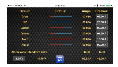
system. It shows you the status of each circuit, the current amperage draw by circuit, total amperage draw, and allows you to adjust the alarm voltage.
