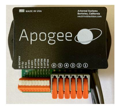
Step 5. Connect up the powered/controlled devices to the large terminals labeled 6 through 1
