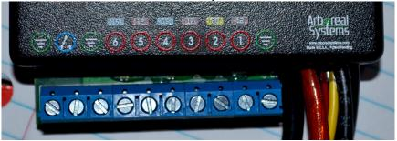
Circuits 1,3, and 5 are each rated at 12 amps, circuits 4 and 6 at 15 amps, and circuit 2 at 20 amps. This is the maximum load that each circuit can handle, and the software won't let you set a level higher than this. This is done to optimize internal electrical paths within the unit.
