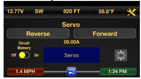
Holding your finger on either the reverse or forward buttons will activate the servo motor in the intended direction. (requires optional servo adapter)
