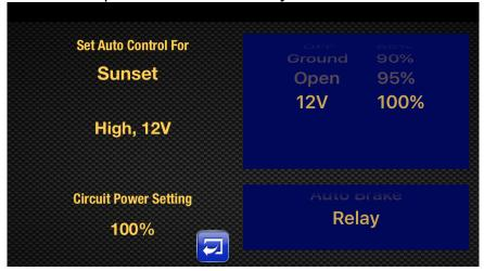
Going back to the previous screen, the next option is circuit breaker level. Tapping this button will bring up a scroll wheel that allows you to disable the circuit or change the breaker level from 2 amps up to the maximum for that circuit.
