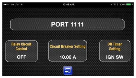
This screen allow you to name the circuit by tapping the circuit name, access the relay control screen, set the circuit breaker limit, and set how the circuit behaves when the ignition is off.
