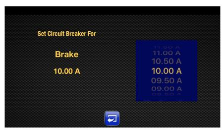
To set circuit the break limit for this circuit simply twirl the wheel to the desired amperage value.
