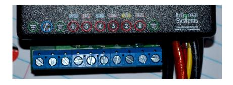
Circuits 1,3, and 5 are each rated at 12 amps, circuits 4 and 6 at 15 amps, and circuit 2 at 20 amps. This is the maximum load that each circuit can handle, and the software won't let you set a level higher than this. This is done to optimize internal electrical paths within the unit.
