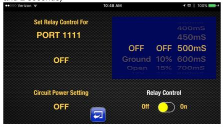
The other option on this screen is setting up relay control. What this does is to use an INPUT to the relay input terminal (2nd from the right on the terminal strip) and allow you to configure any number of circuits to activate or deactivate using this input.
