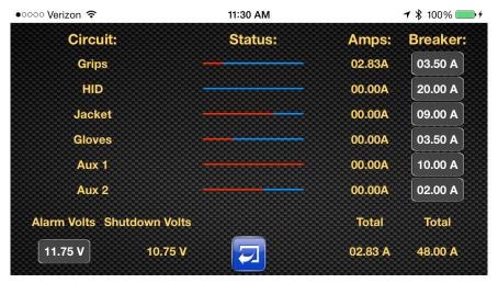
Here you can see the realtime status of each circuit, the current amperage draw by circuit, total amperage draw. You can also adjust the alarm voltage.
