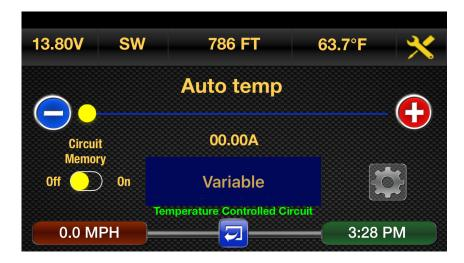
restart. If set to the "on" this circuit will return to the state it was in when the system was last shut down. Very
