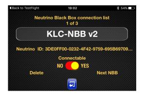
Note: your phone must be "connected" to Element in order to program the module. Settings are saved when the ignition is shut off. If you shut down the app before the ignition, settings won't be saved.
