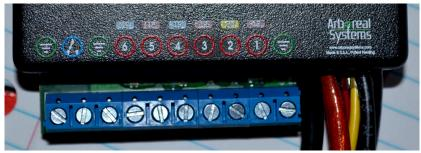
Note on grounding. Element includes a ground plane. This allows you the flexibility to take ground from either the Element module or from the chassis. This not only greatly simplifies installation, but it also allows for direct connection of sensitive audio equipment without the risking ground loop issues resulting from the use of chassis ground.
